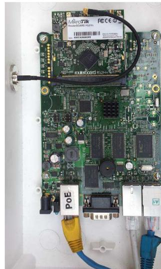
Fig.14. RouterBoard RB433
