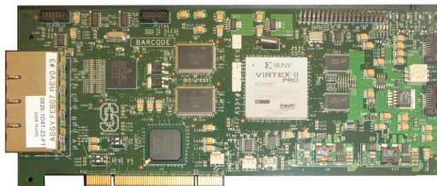
Figura 1. NetFPGA de 1Gbps. Tomado de [http://netfpga.org/1G\\_specs.html](http://netfpga.org/1G_specs.html)
